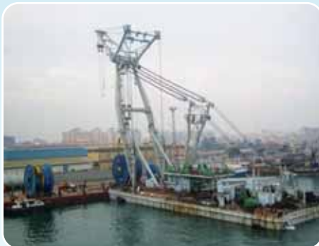
A floating crane lifts the full reels onto the construction vessel.
