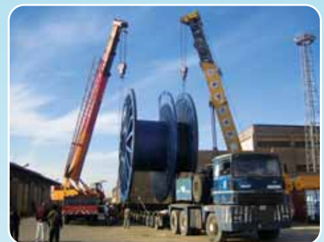
Master-slave mobile cranes discharge the reels in the storage yard.
