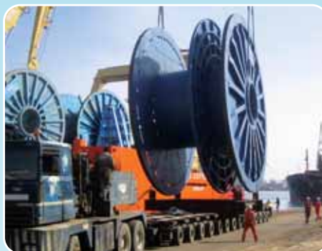
An empty reel is adjusted on the transport frame of the low loader provided by GAC Egypt.
