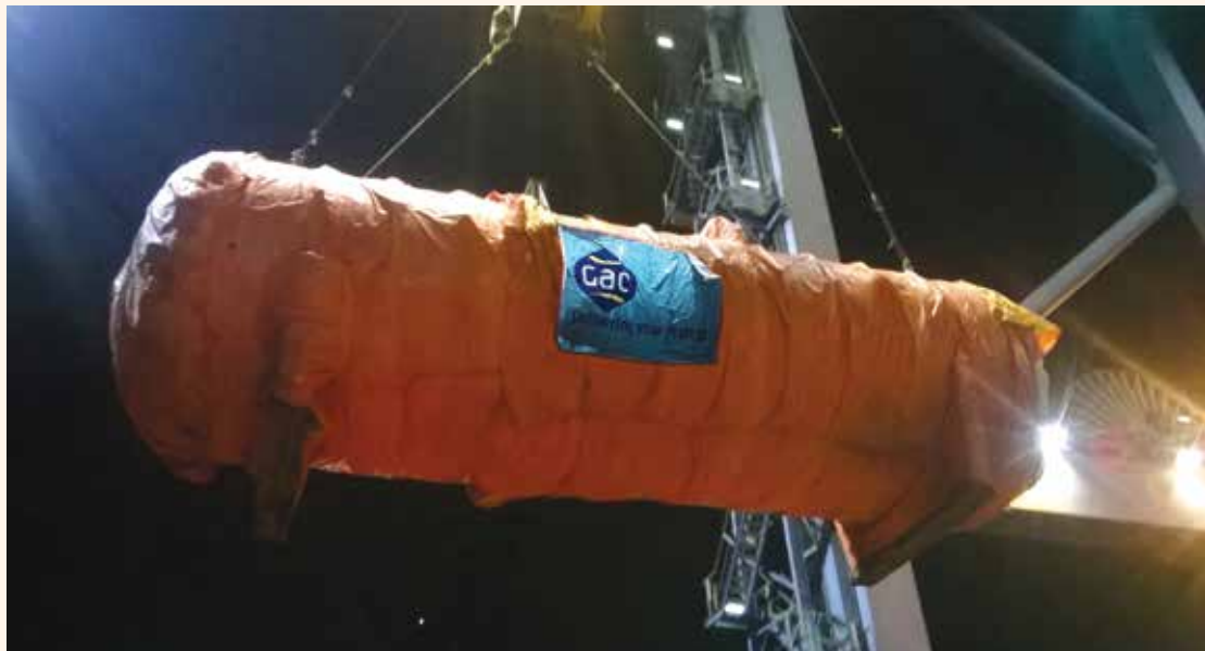
Lifting of the supersized boiler as breakbulk cargo on a container vessel.
